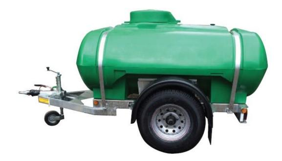
**CHASSIS:** Constructed from 5mm pressed steel section fully welded with a front standing plate and 100 x 50 RSC 'A' frame drawbar.
