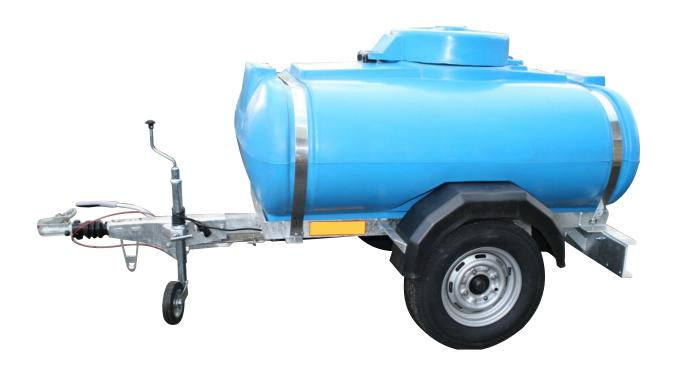
**CHASSIS:** Constructed from 80 x 80 RSA. fully welded with a 'T' frame drawbar, all fully hot dipped galvanised to B.S. Standards.
