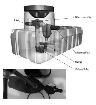
Connect the supplied right angled connector to the top of the vertical pipe. Attach the remaining length of hose to the right angled connector and feed it to the house through a Ø110mm service pipe. Use PTFE in all connections after the pump (but not before) to ensure a pressure tight system. Most water company inspectors now require rainwater pipe to be black with green stripes. Ensure no pipes are exposed to the cold when ducted to and inside the building.
