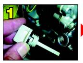
Fill engine with oil to correct level
