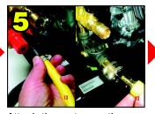
Attach the water suction hose to the machine inlet connection
