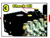
Check the oil levels for the pump, and gearbox (if fitted)
