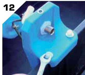
12 Tighten using a 13mm spanner.
