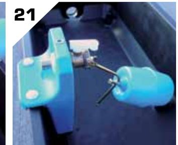
21 Once tightened bring the float valve back to its vertical alignment position and secure the ballcock cover again.
