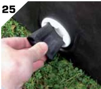
25 Using the plug key provided unscrew the plug and allow the water to drain.
