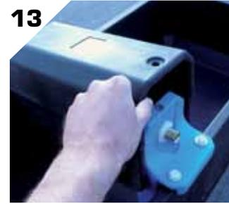
13 Position the ballcock cover over the ballcock support.
