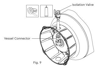
e) The vessel assembly should then be positioned and checked to ensure there is sufficient space to install the upstream line-in kit between the stopcock and pressure vessel inlet. Refer to the chart (Fig. 17) as a guide.
