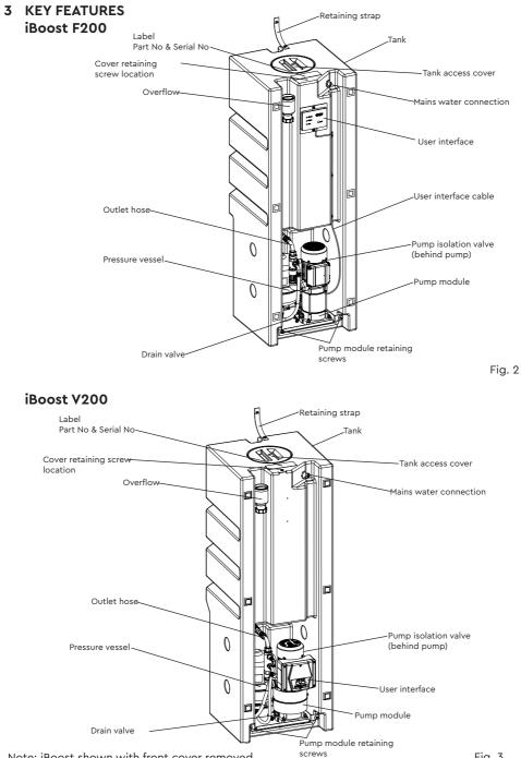
Note: iBoost shown with front cover removed
