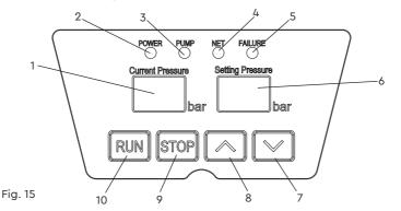
Note: The maximum pressure this unit can generate is 4.5 bar. **Do not** set the pressure required above 4.0 bar.
