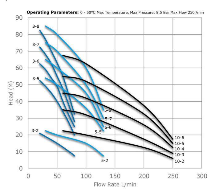
All systems set at mid curve efficiency during first activation on wet test using the RS variable speed inverter at closed valve up to max pressure. The performance curves are based on kinematic viscosity values = 1/mm2/s and density equivalent to 1000kg/m3.
